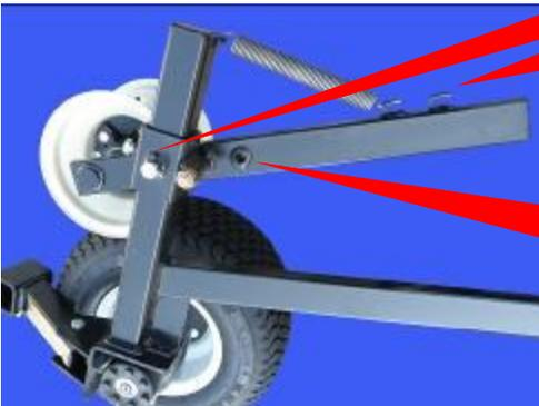
Loosen bolt to adjust the wheel to tile size. Move spring to best fit for tile size.
