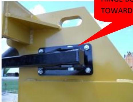
**Step Two:** Install the hydraulic hose holder.
