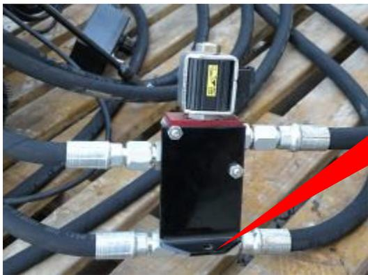
Hoses are preset and tested at shop for correct operation. Switch hoses at the tractor remote if wheel is moving in reverse, do not change hoses at the proportional valve or at the motor.
